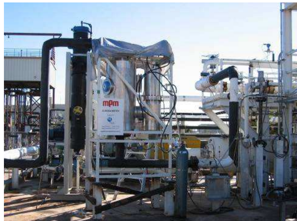
Picture of a 5" MPM Subsea meter tested at SwRI, San Antonio, Texas
