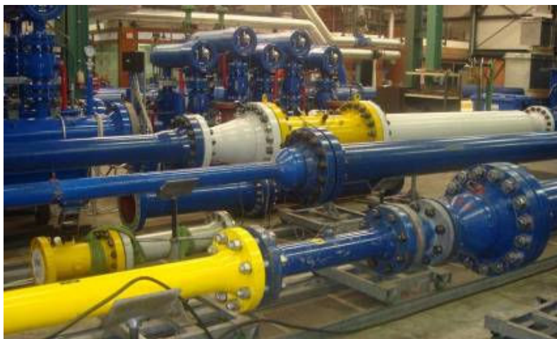
Fig. 23 Typical pipe size reduction at a flow calibration lab (photo courtesy of NMI)
