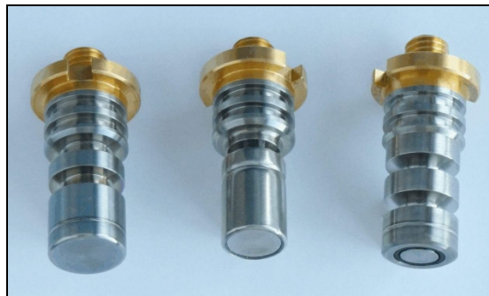
Figure 3: Ultrasonic transducer with different operating frequencies (80 kHz, 135 kHz, 208 kHz)
