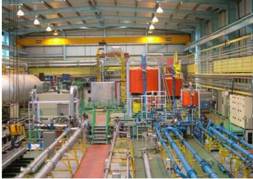
Figure 2 The NEL oil (blue, right) & water (silver, left) calibration facilities
