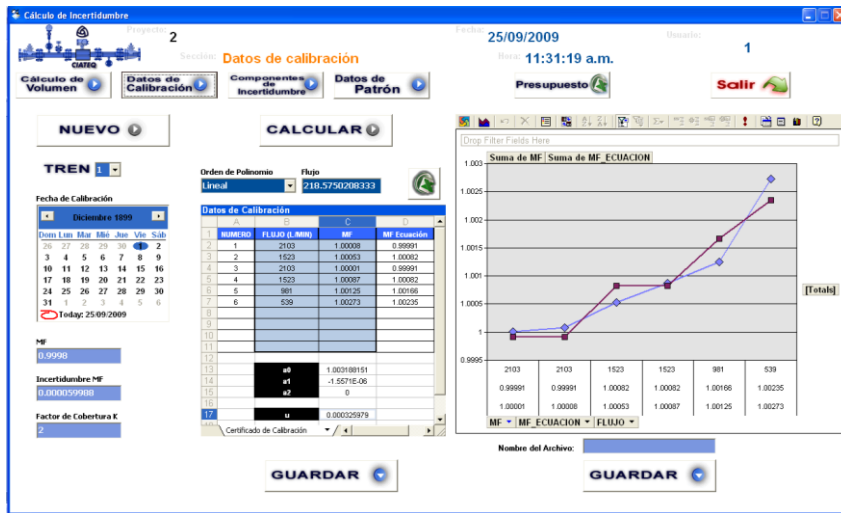
Figure 6. Calibration curve and its associated uncertainty screen
