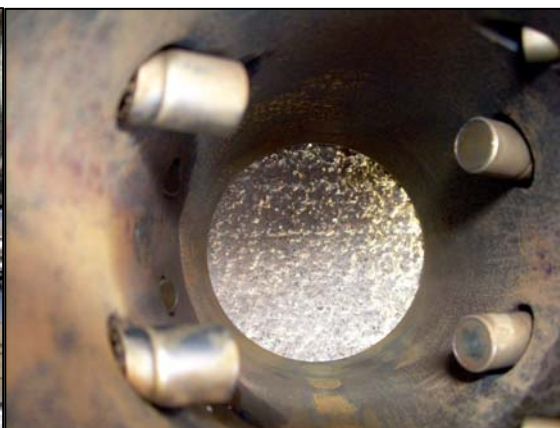
Figure 3 – Transducers in the 4+2 Meter
