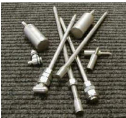
Fig. 14 A variety of ultrasonic transducers, at different frequencies, are used in flare gas flow measurement.
