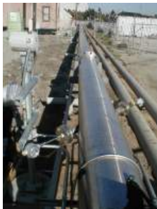
Fig. 20 This installation is on a 14 inch pipe, with a 19 inch path. In 100% pure CO2. Temperature is ambient and pressure approximately 30 PSIA. Plot of freq/pressure = 0.05 with a 100 kHz transducer is shown.
