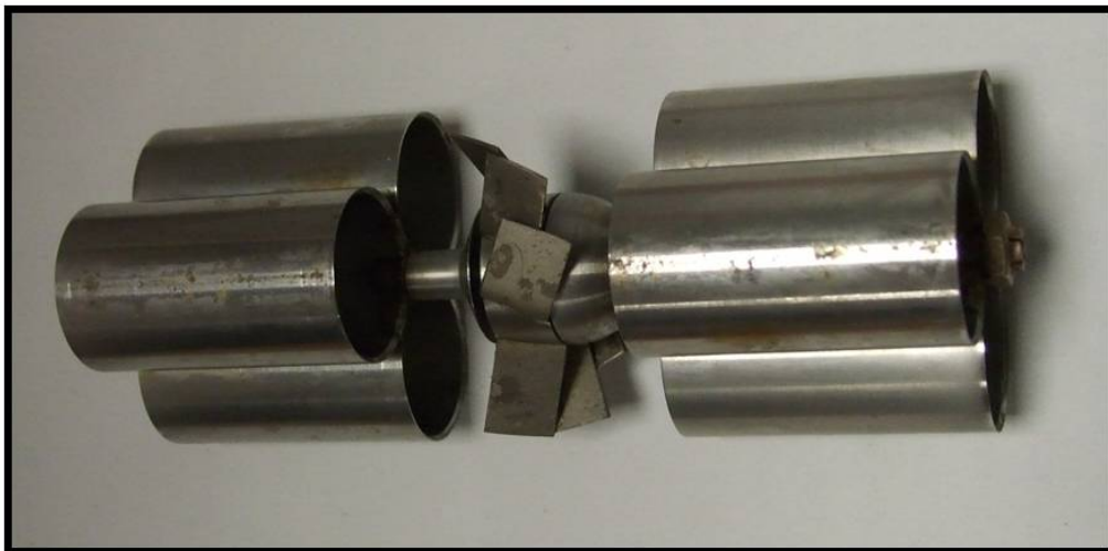
Figure 3: Turbine meter with damaged blades
