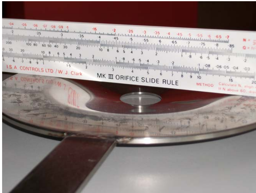
Figure 2: Bent orifice plate
