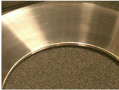
Fig.33 Photograph of worn orifice edge worn, 3 DP's.
