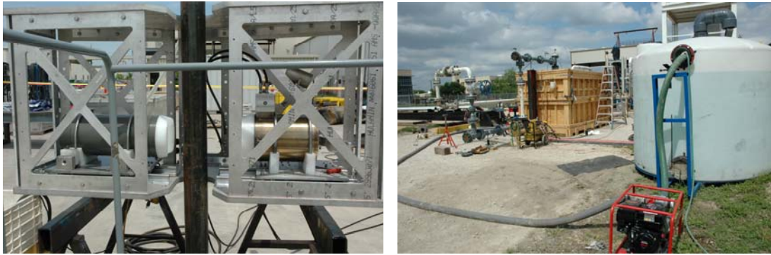
Figure 6. On left, marinized ROV-conveyed Neftemeter meter in delivery frame. Flow test setup at SwRI shown on right, with wooden tank for submersion of meter during tests.
