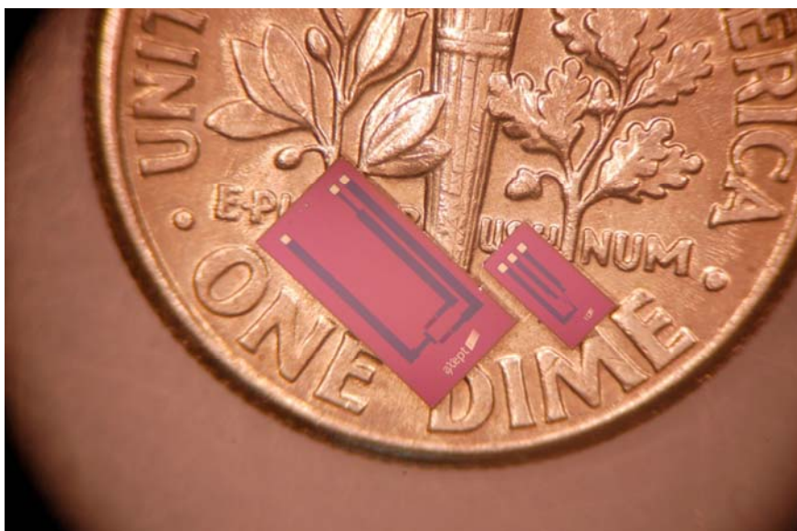
Figure 7. HP/HT differential and line pressure sensor prototypes
