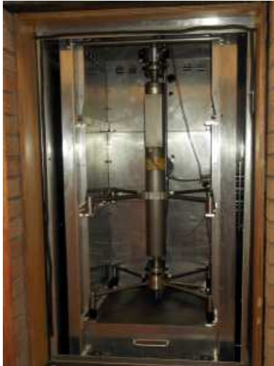
Figure 25:- The NEL Primary Density Calibration System with S/N 352825 installed
