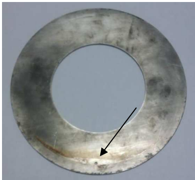
Figure 1:- Orifice Plate with Drain Hole Indicated
