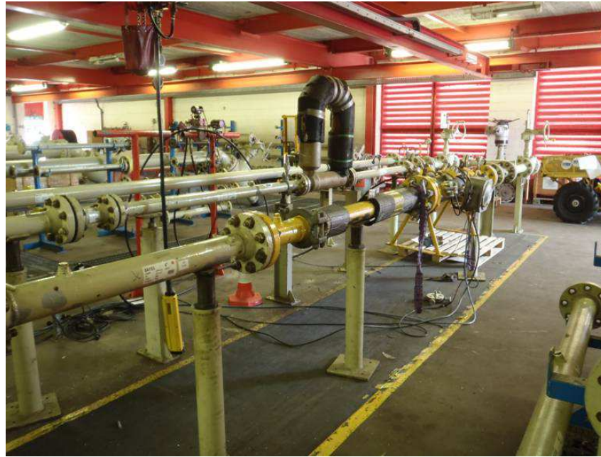
Figure 9:- Banff FPSO Export / Injection Meter Calibration Set-Up
