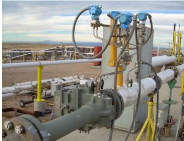
Fig 16. 4",sch 40, 0.62 \beta orifice Fig 17. 4",sch 80 0.6 \beta Venturi Fig 18. 4",sch 80 0.75 \beta cone
