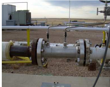
Fig 16. 4",sch 40, 0.62 \beta orifice Fig 17. 4",sch 80 0.6 \beta Venturi Fig 18. 4",sch 80 0.75 \beta cone
