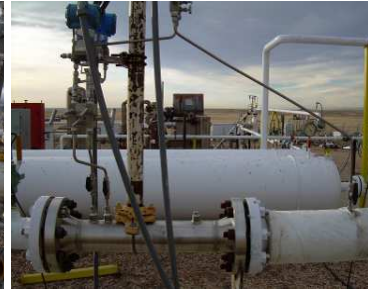
Fig 16. 4",sch 40, 0.62 \beta orifice Fig 17. 4",sch 80 0.6 \beta Venturi Fig 18. 4",sch 80 0.75 \beta cone
