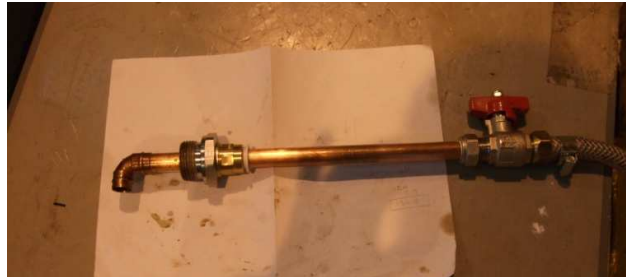
Figure 2: Sampling probe for water-in-oil research
