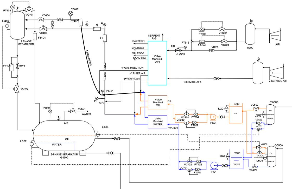
Fig. 3 - Cranfield University Multiphase Loop showing 101.6mm Catenary Riser and 50.8mm Vertical Riser (Cao and Yeung, 2009)
