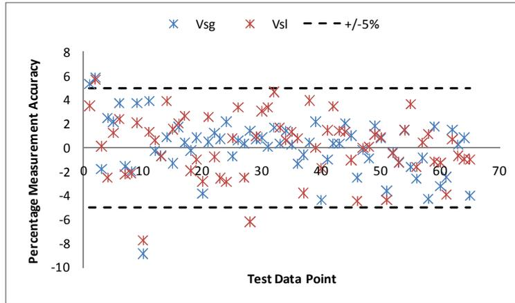
Fig. 6 - Prediction Performance from the Soft Energy Gamma Features (50.8mm Flow Loop Data)
