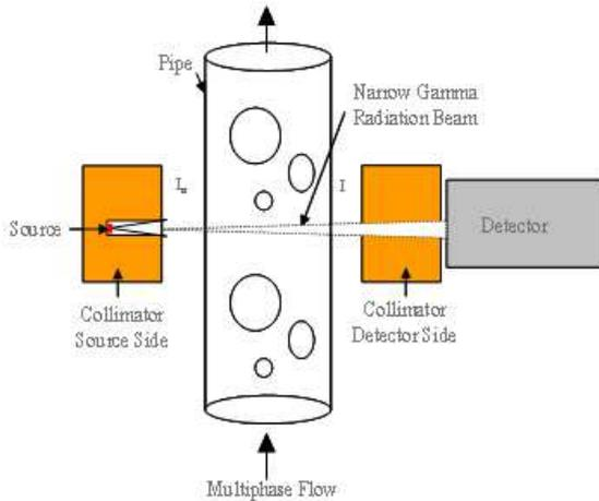
Fig. 1 - Gamma Densitometer (Arubi and Yeung, 2010)
