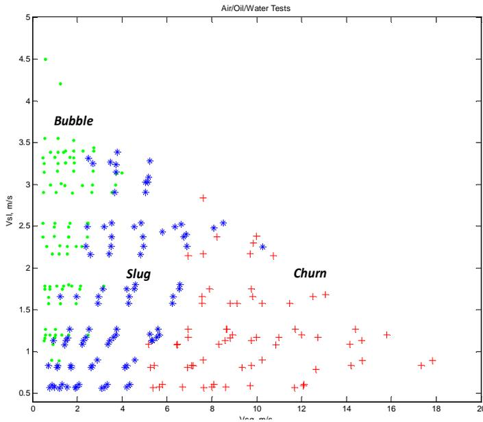
Fig. 4 - 50.8mm Flow Loop Vertical Regime Map for Three Phase Tests
