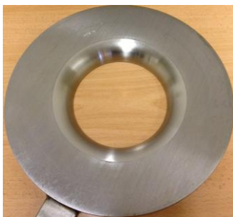
Figure 4 8 inch \beta 0.6 Quadrant Edge Orifice Plate Inlet
