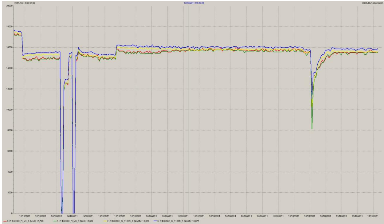
Figure 16 – Respective measurement of the clamp-on meters and downstream meters, K12-C
