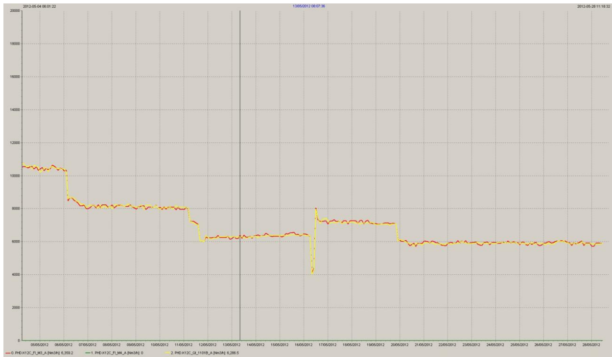
Figure 17 - Outputs of clamp on ultrasonic meter (well 4) and reference meter, K12-C
