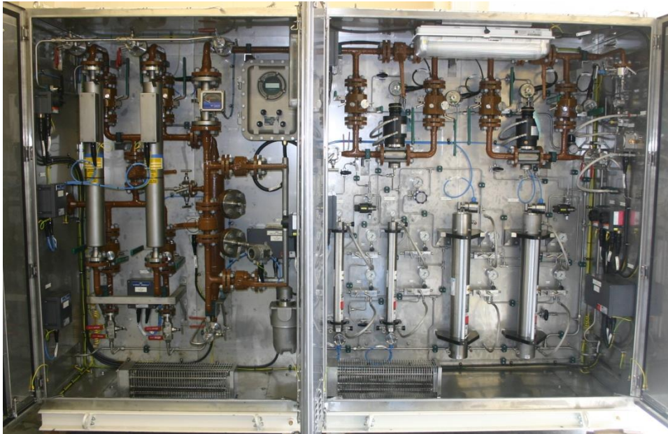
A typical quality system for use on high RVP oils including cell samplers, CPC receivers, density meters, OWD. (Part of a CoJetix system)
