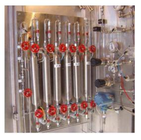
Figure 5 Example of gas sample containers [Courtesy of Enagas]
