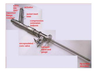
Figure 2 Vacuum insulated LNG sampling probe with connection line to vaporiser [9]
