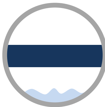
Figure 11: Illustration of the blocking effect of water hold-up on the actual velocity perceived by the meter.
