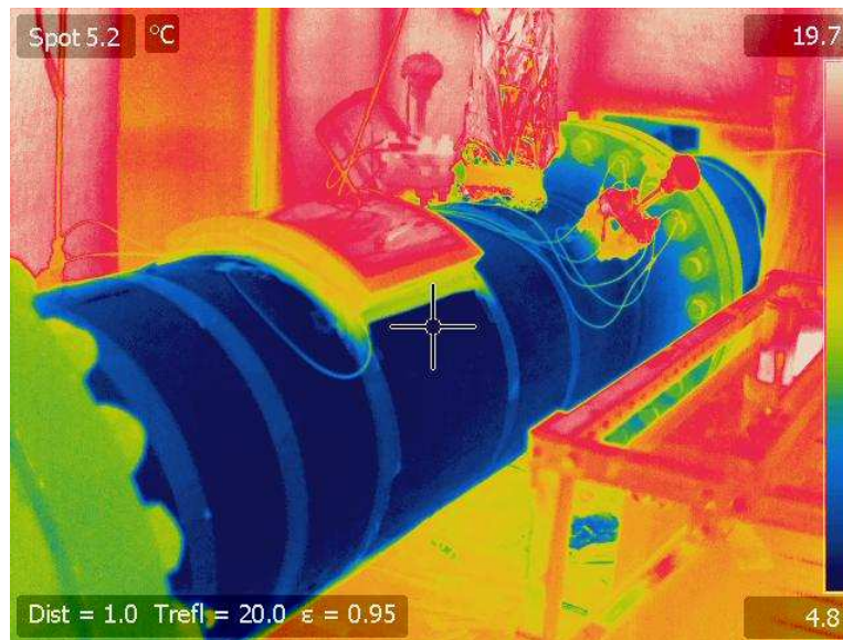
Fig. 24 – 24-inch spool during high temperature tests
