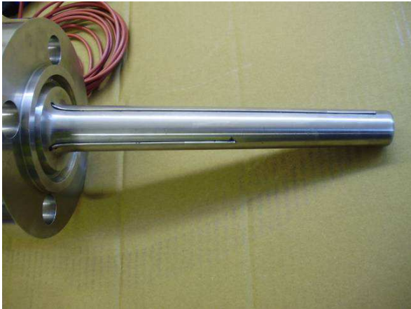
Fig. 13 – Pictures of actual thermowells installed for tests
