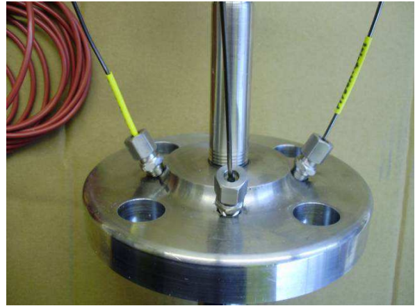
Fig. 13 – Pictures of actual thermowells installed for tests
