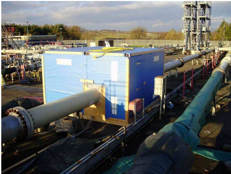
Fig. 19 – Environmental test enclosure installed on the 24 inch test pipe at a DNV GL Flow Centre
