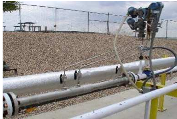
Fig 18. 2” Venturi Meter Multiphase Wet Gas Flow Tests.
