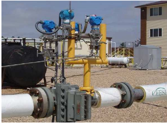
Fig 9. 4" Dual Chamber Orifice Meter Multiphase Wet Gas Flow Tests at CEESI.
