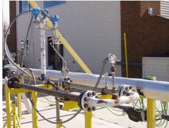
Fig 10. 2" Paddle Plate Orifice Meter Multiphase Wet Gas Flow Tests at CEESI.
