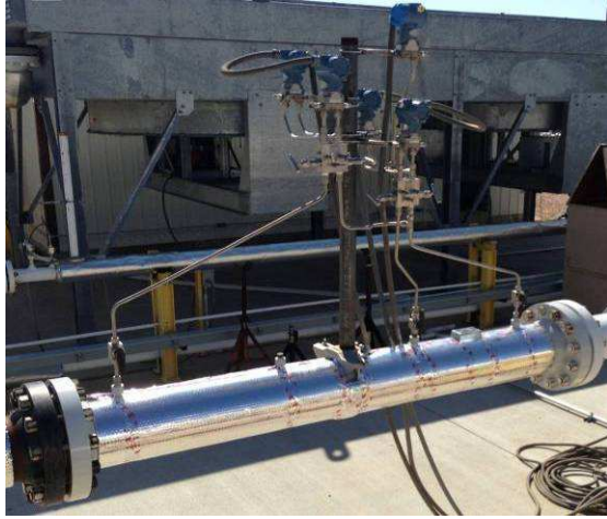
Fig 15. 8” Venturi Meter Multiphase Wet Gas Flow Tests.
