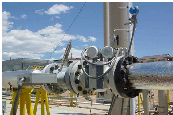
Fig 30. 8" Four Chordal Path Ultrasonic Meter at the CEESI Wet Gas Test Facility
