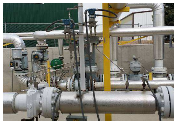
Fig 12. 8" Dual Chamber Orifice Meter Multiphase Wet Gas Flow Tests at CEESI.
