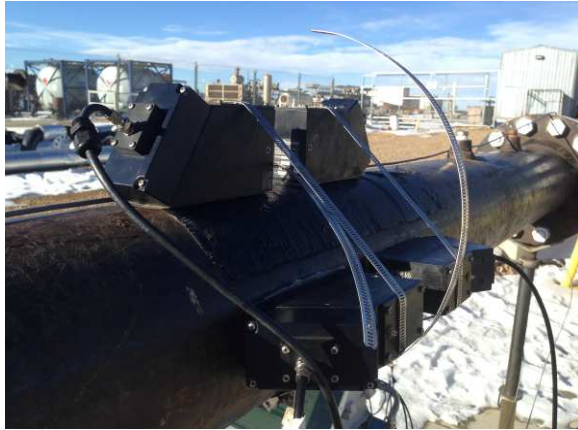
Fig 25. Clamp On Ultrasonic Meter Under 8” Wet Gas Flow Tests at CEESI
