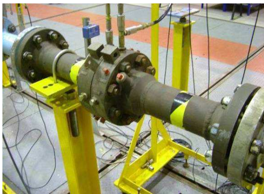
Fig 11. 4" Paddle Plate Orifice Meter Two-Phase Wet Gas Flow Tests at TUVNEL.
