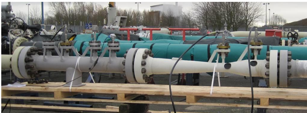
Fig 13. 8”, 0.4 Beta Ratio Venturi meter Under Calibration
