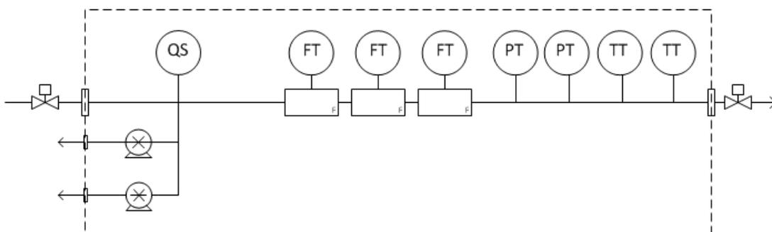
QS = Sampling System, FT = Ultrasonic Flow Meter, PT = Pressure Transmitter, TT = Temperature Transmitter.
