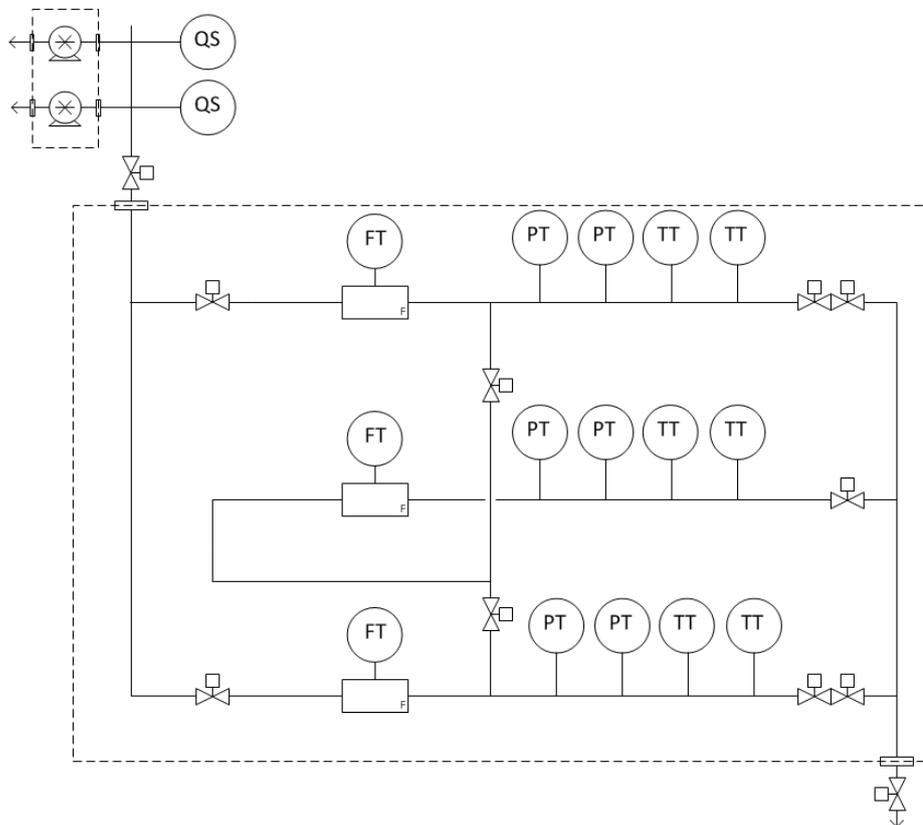
QS = Sampling System, FT = Ultrasonic Flow Meter, PT = Pressure Transmitter, TT = Temperature Transmitter.
