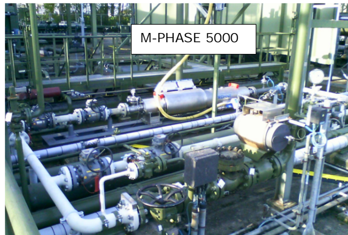
Figure 2: The magnetic resonance multiphase flowmeter (M-PHASE 5000) installed in a field test by a Dutch exploration and production company on a production location in the Netherlands.
