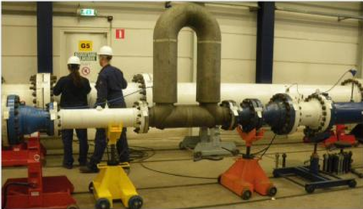
Fig.3. Coriolis Meter Installed for Independent Gas Laboratory Testing 4
