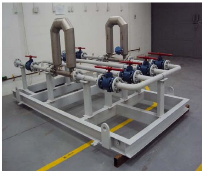
Fig.2. Trial skid with Two Micro Motion CMF200 Meters
