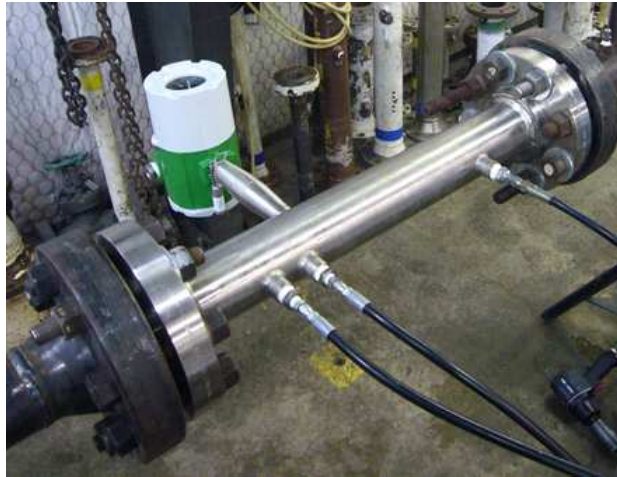
Fig 35. 3" 0.68β Hybrid Vortex / Cone DP Meter Under Air Flow Testing at CEESI.
