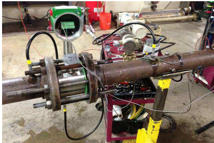
Fig 18. The Prototype Mass Meter Installed at CEESI.
