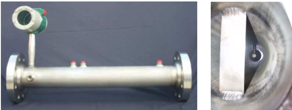
Fig 8. First 4" Prototype Mass & Volume Flow Meter and Densitometer
