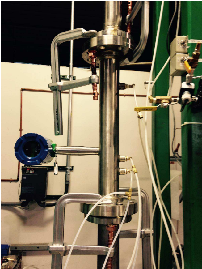
Fig. 31. 3" 0.68 \beta Meter Drawing & a 2", 0.5 \beta at Vortek Water Facility
