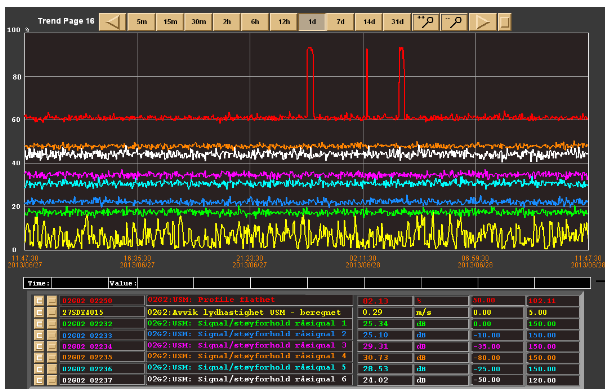
Fig. 6.5.1-1: Change of profile flatness during periods with peaks compared with SOS and signal to noise ratio
