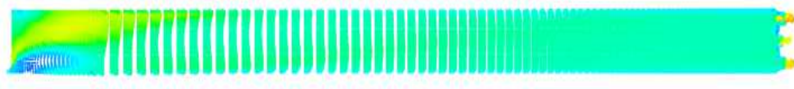
Figure 2.8 Flow velocities in run 1 single operation between the manifold and the modified position of the CPA-plate. The vectors are shown in a horizontal plane through the meter pipe axis. Similar plot as Figure 2.5, but with flow conditioner 3.8 m after the manifold.
