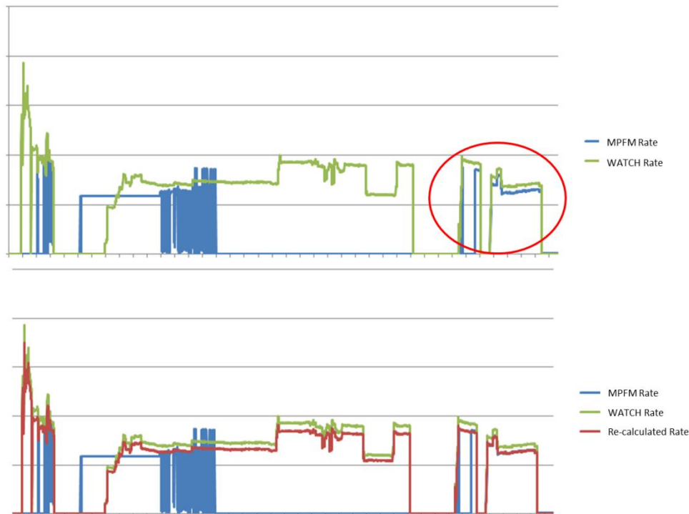
Figure 11 The top figure shows the WATCH as an online tool where WATCH was used as the primary measurement. The red circle shows when the MPFM came online. The bottom figure shows flow rates prior to and after calibration.
