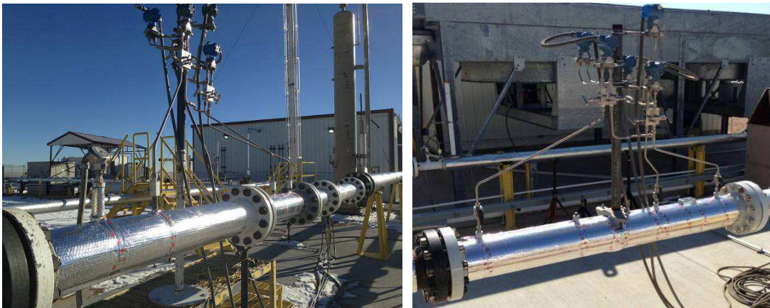
Fig. 13 - 6" (left) and 8"(right), 0.6 \beta Venturi Meter at CEESI
