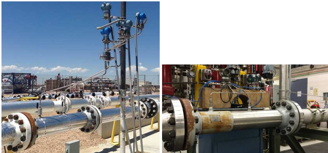
Fig. 5 - 6", 0.6 \beta Venturi meter at the CEESI (left) and DNV GL(right) wet gas test facility
