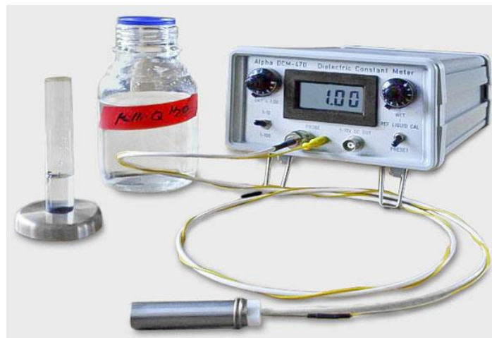
Figure 14 Oil permittivity instrument “Alpha DCM-470”
