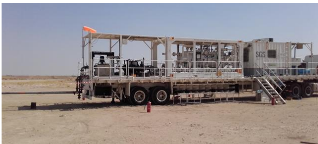
Figure 8 SGS mobile test separator used as a reference measurement system.
