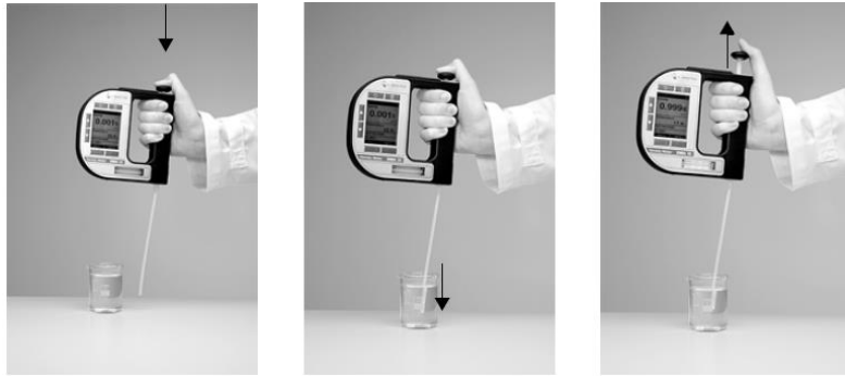
Figure 15 Illustration of the density measurement by Anton Paar DMA 35 Handheld densitometer
