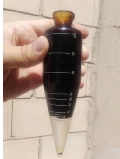
Figure 11 Left: L-K Industries Melton Oil Centrifuge for field applications, right: a centrifuged oil-water sample from KOC well in a ASTM D91/D96 tube.
