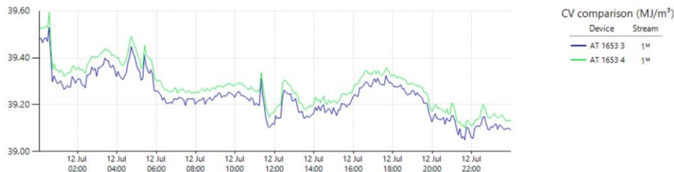
Figure 28. CV comparison between two GC from 12/7/2017
