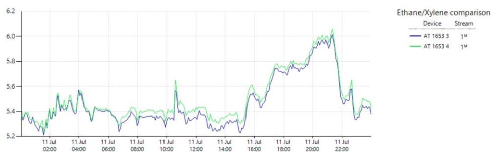
Figure 30. Ethane drift on GC A
