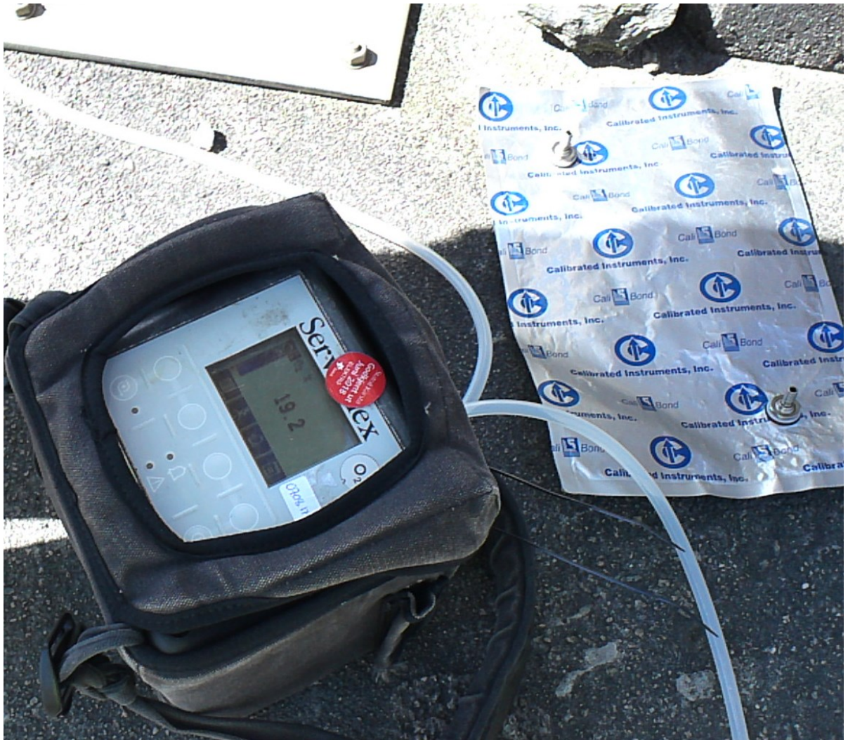
The picture shows the Servomex O 2 -analyser and the sample bag.
