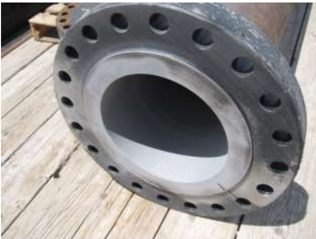
Figure 4. Roughened (500 μ-in) Meter Tube Inlet
