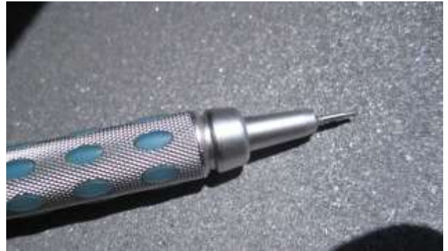
Figure 5. Close-up of Roughened Meter Tube (mechanical pencil in foreground for scaling)
