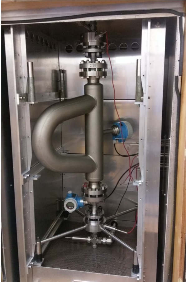
Figure 7: Test installation of Promass Q 500 DN50 (top) with Cerabar S PMP71 pressure transducer (bottom) vertically mounted in NEL's temperature-controlled chamber.
