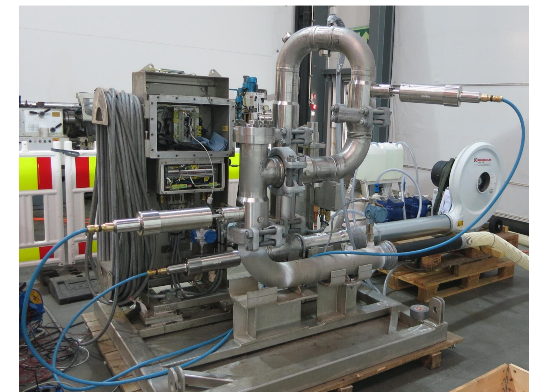
One-pass flow rig for testing MEG-water measurements
