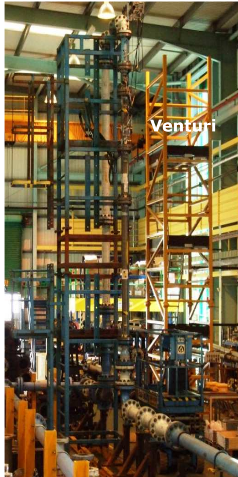
Figure 11 Photographs showing the installation of the Venturi directly after a blind-T and with 30D straight upstream pipe (tested in 2014).
