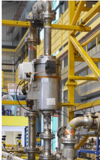
Figure 2: M-Flow Multiphase Fraction Meter Under Test at NEL Flow Loop
