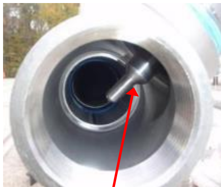
Probe Inserted 3-4" into Pipe
