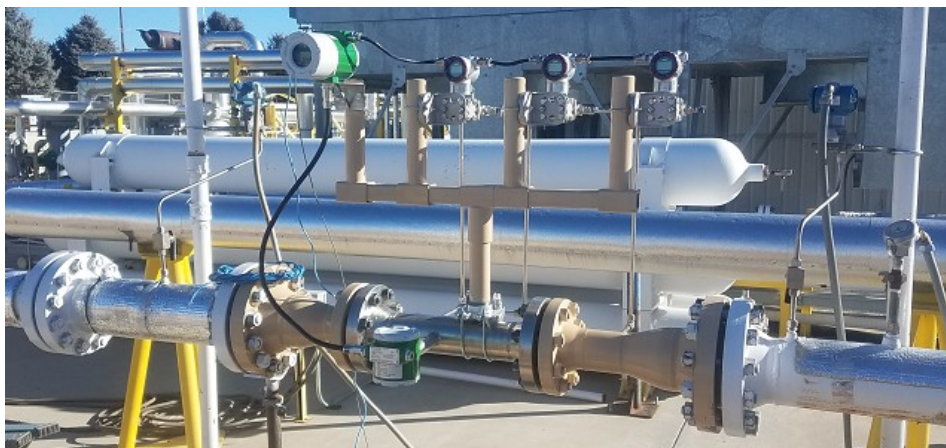
Figure 10. 6" to 4", 0.75 \beta VorCone Meter at the CEESI Natural gas Facility.
