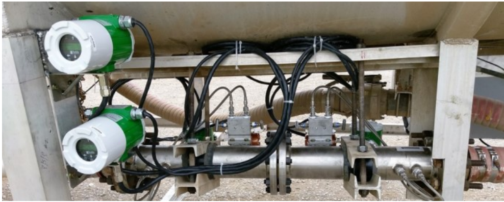
Fig 13. Oil Truck Mounted 4" VorCone Meters (One per Flow Direction).
