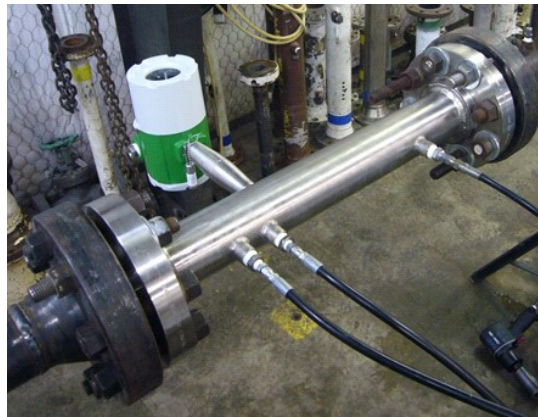
Fig 7. 3", 0.68 \beta VorCone Meter During Air Flow test at CEESI.
