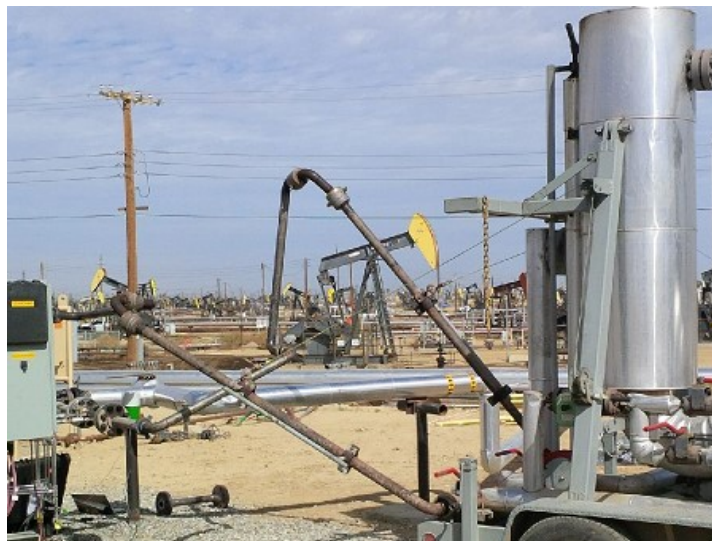
Fig 16. Saturated Steam Portable Cyclone Separator Reference System at Well Head.
