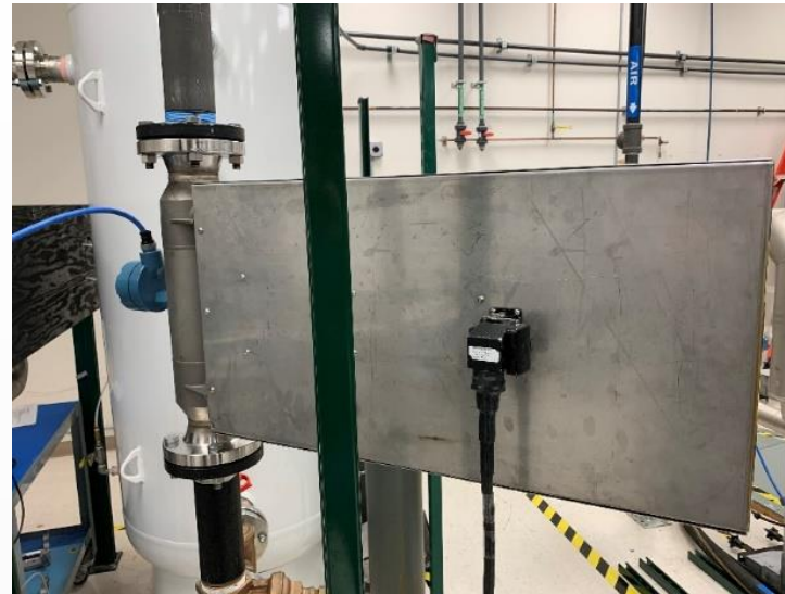
Prototype Speed-of-Sound Augmented Coriolis Meter
