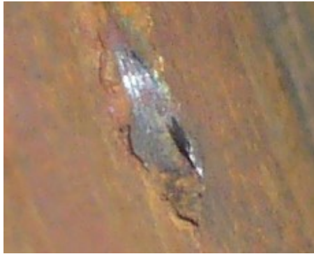
Fig 46. Venturi Pressure Port Burr.
