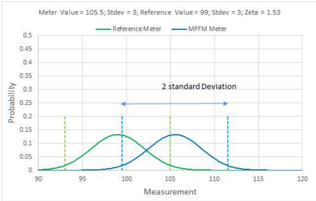
Figure 8: Comparison permanent flowmeter vs. reference flowmeter with a \zeta -score of 1.53
