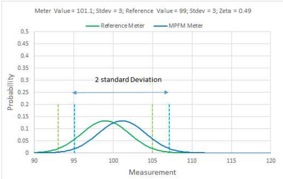
Figure 9: Comparison permanent flowmeter vs. reference flowmeter with a \zeta -score of 0.49
