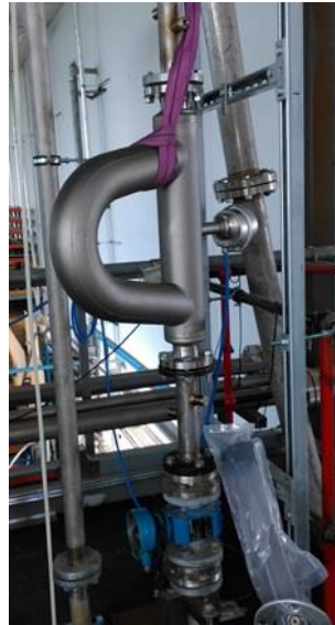
Fig. 3 – Meter Under Test in “Flag” Position
