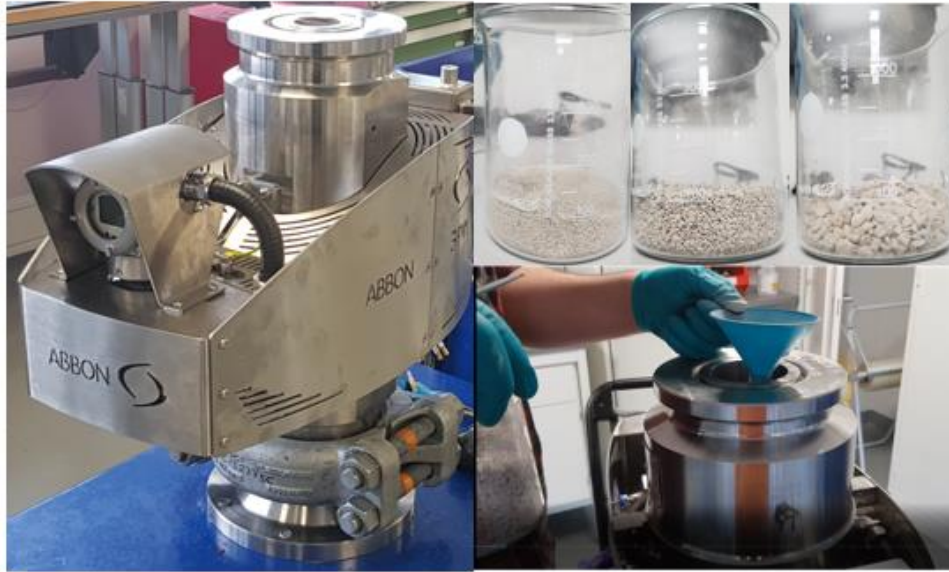
Figure 4. Set up for the impedance sensor sensitivity test around solid particles in fluid phase.
