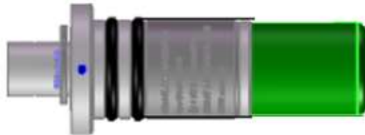
Figure 8: The epoxy/SS transducer.
