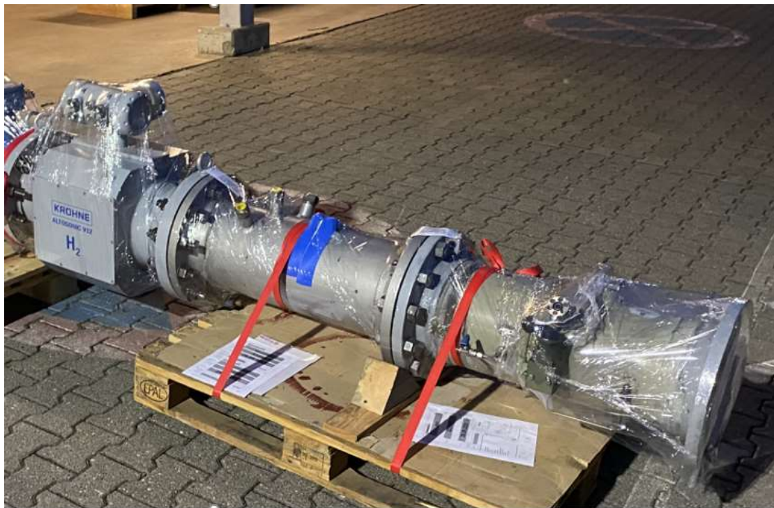
Figure 4: The 10" ALTOSONIC V12 custody transfer gas flowmeter including meter run as supplied to Pigsar for calibration.
