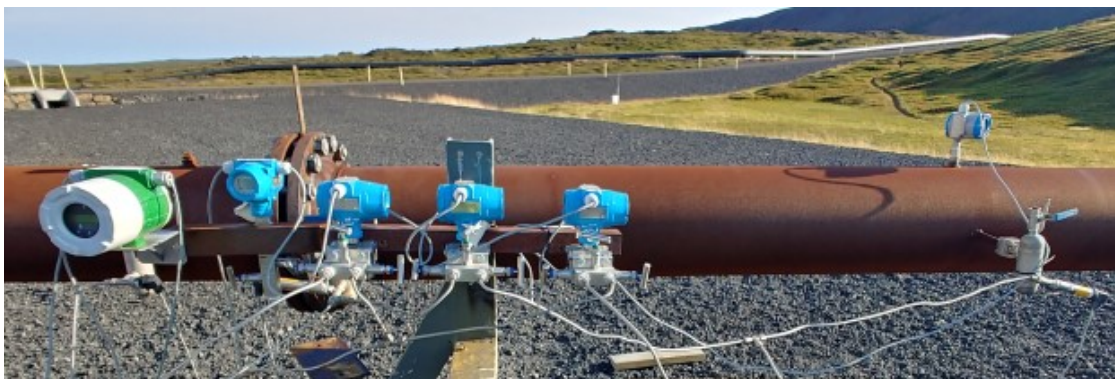
Fig 13. 14", 0.48 \beta Orifice Meter with Instrumentation.
