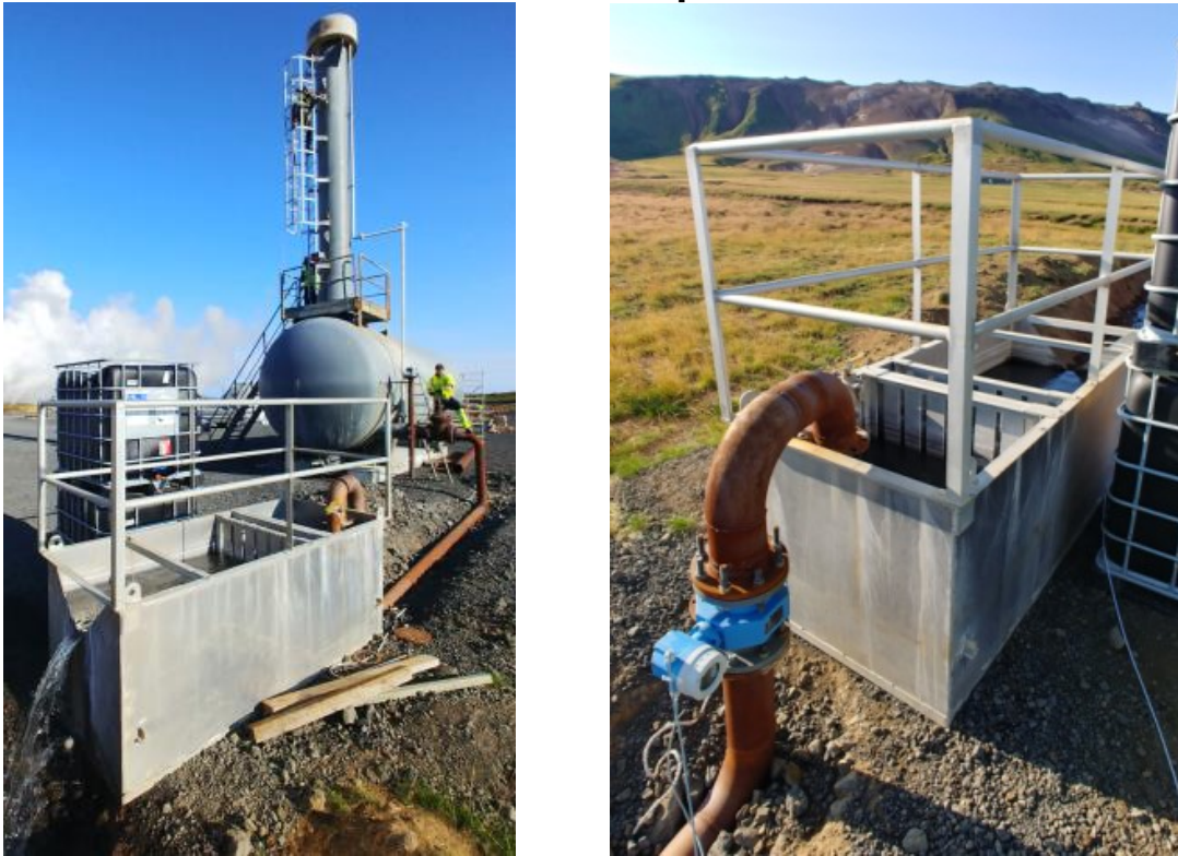
Fig 11. Magnetic Meter and Weir Separator Discharge Reference Water Flow System.
