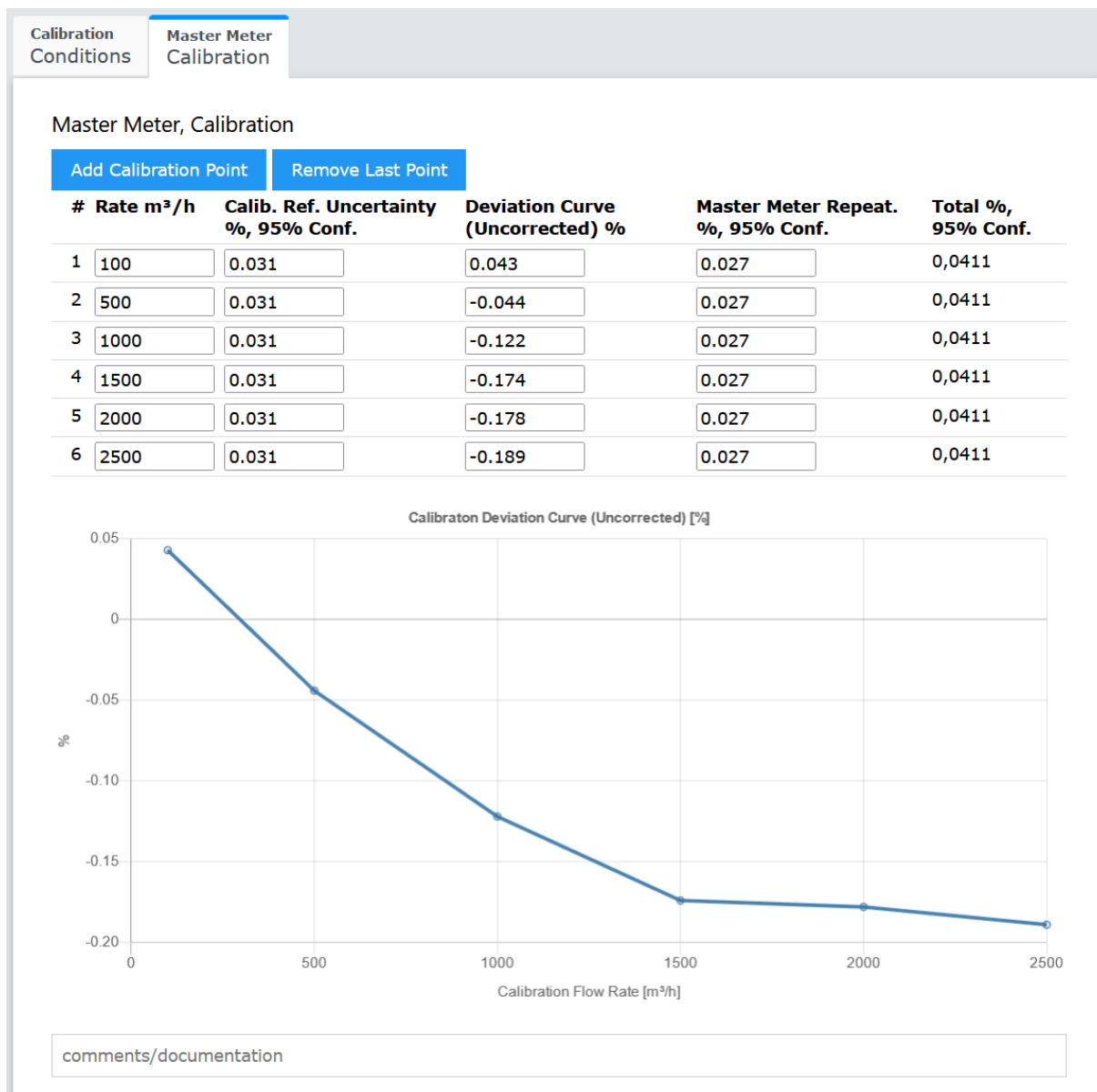
Figure 6.10. “Calibration”-page with “Master Meter Calibration”-section selected. This page concerns calibration conditions and uncertainty in the calibration procedure.
