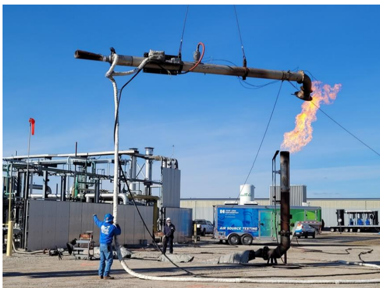
Figure 4 the flare.IQ extractive sampling testing at John Zink, Tulsa, OK
