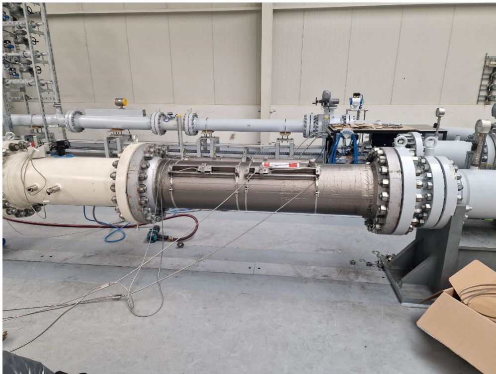
Figure 17 Flexim meter installed in the loop; in the background the sound speed reference meter
